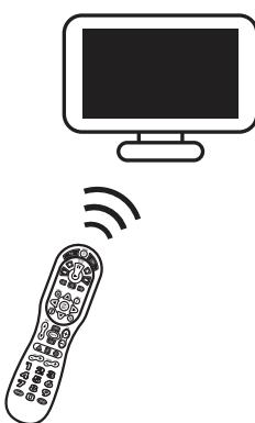
**4** Press the power button to test TV control. If the TV turns off, setup is complete.
